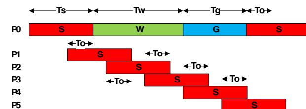
$$\text{进程数的计算: } N = 1 + \left\lceil \frac{T_w + T_g + T_o}{T_s - T_o} \right\rceil$$
